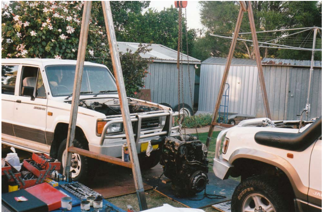
4JB1 engine after removal:
